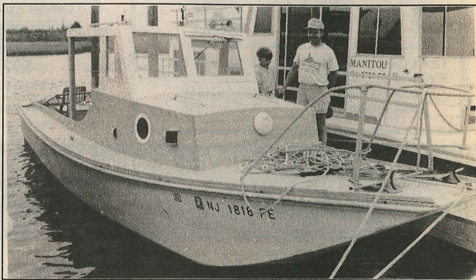
The Gail was designed as a clamming boat, able to go into shallow waters.
